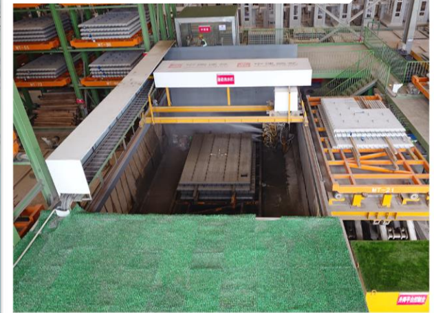
Concrete Surface Clearing done by Robots
