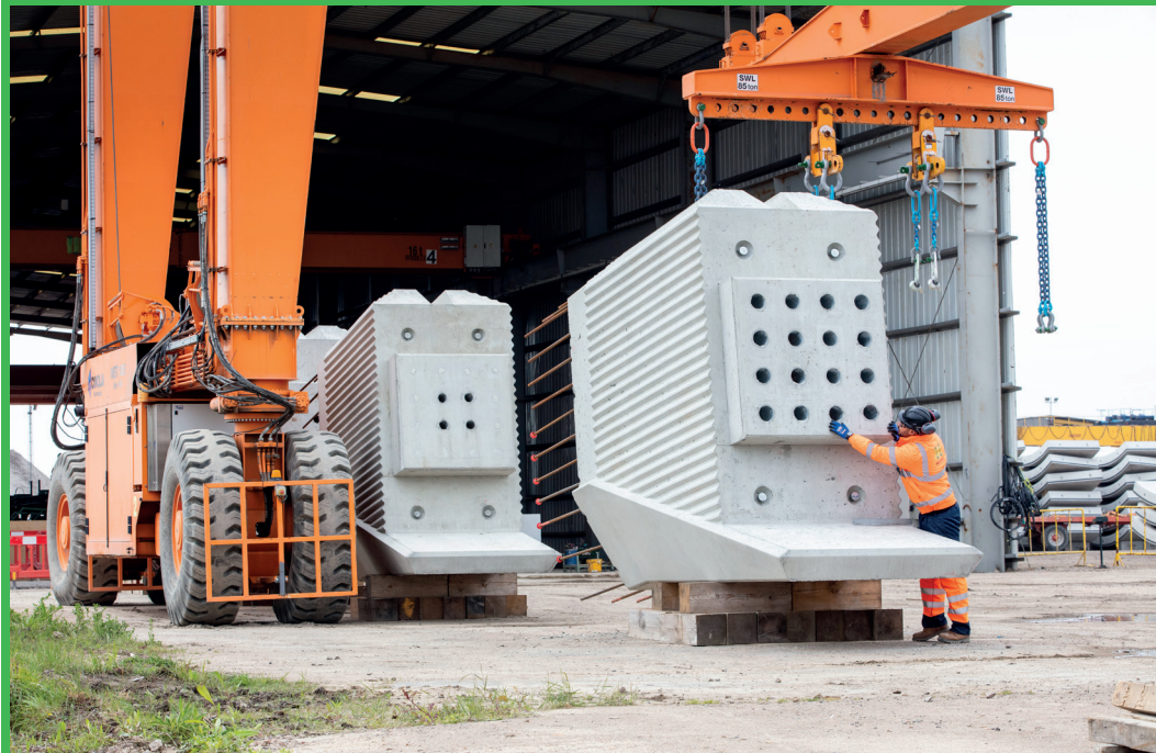
Figure 11 Completed piers for the Thame Valley Viaduct at the Pacadar UK factory (courtesy HS2 Ltd)
