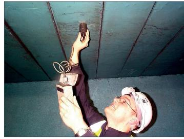
Figure 3 Testing precast beams shows a cover survey being undertaken on precast concrete beams
