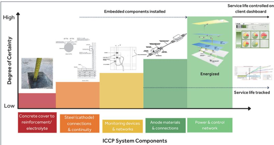
Figure 19 Levels of corrosion protection and control. Incorporating ICCP components into new constructions increases confidence that corrosion is controlled for the whole life of the structure
