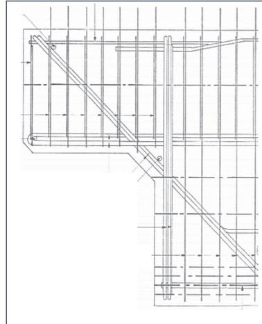
Figure 21 Cross-sectional detail of steel reinforcement arrangement within the half-joint
