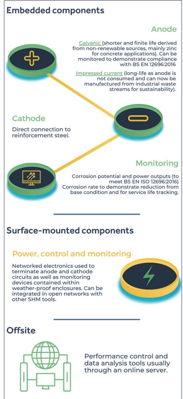
Figure 12 Components of a designed cathodic protection system
