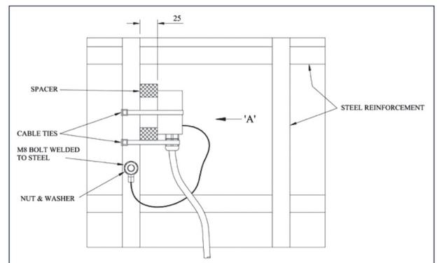
Figure 16 Corrosion rate probe detail (courtesy C-Probe)
