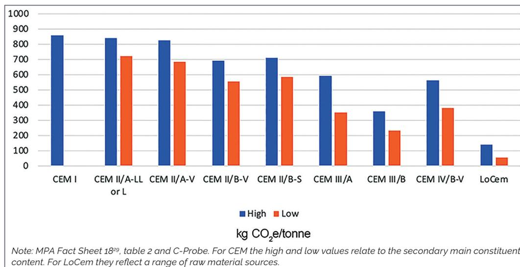
Figure 11 Benchmarking embodied carbon in LoCem (an AACM) used in ICCP systems
