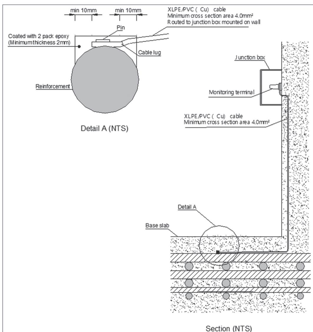
Figure 14 An example of a design incorporating circuitry to link cathodes in a future ICCP system (courtesy Mott MacDonald)
