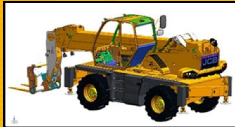
1998 - JCBs trial number 1 of the Rotating Telehandler mocked up by the R&D team.
