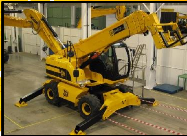
2012 - JCBs trial number 2 of the Rotating Telehandler mocked up by the R&D team.
