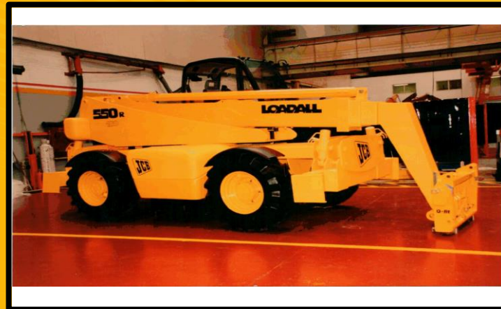
1998 - JCBs trial number 1 of the Rotating Telehandler mocked up by the R&D team.
