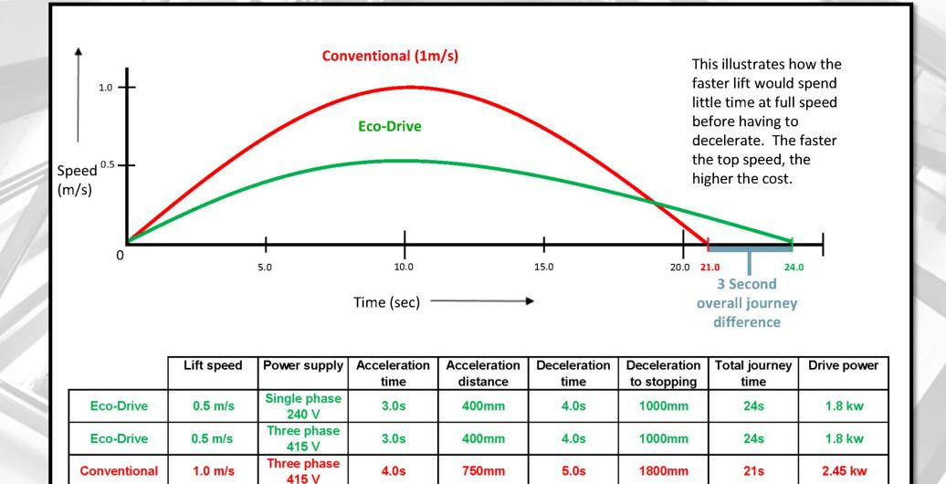
Illustration above based on an IL4 8 person (630kg) traction (MRL) over 4 floors
