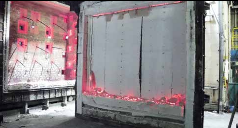
Above: Metrology measurements to assess dimensional accuracy for height of sample module Below: Sample wall panel being removed from furnace after fire test
