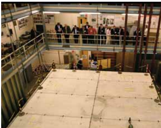
Photos courtesy of GSK Example 4 – Precast concrete deck with steel frame and connectors
