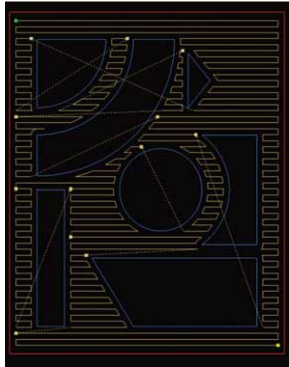
2D 'slice' through sample panel showing tool paths
