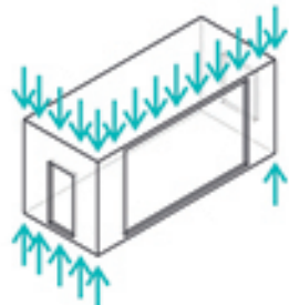
Load paths through corner columns to allow maximum sized openings.
